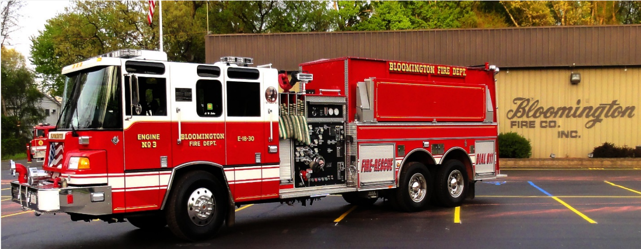
E-18-30 – 1998 Pierce Quantum Pumper / Tanker / 8 passenger cab / 500 gal/min Waterous pump, 2500gsl water tank
