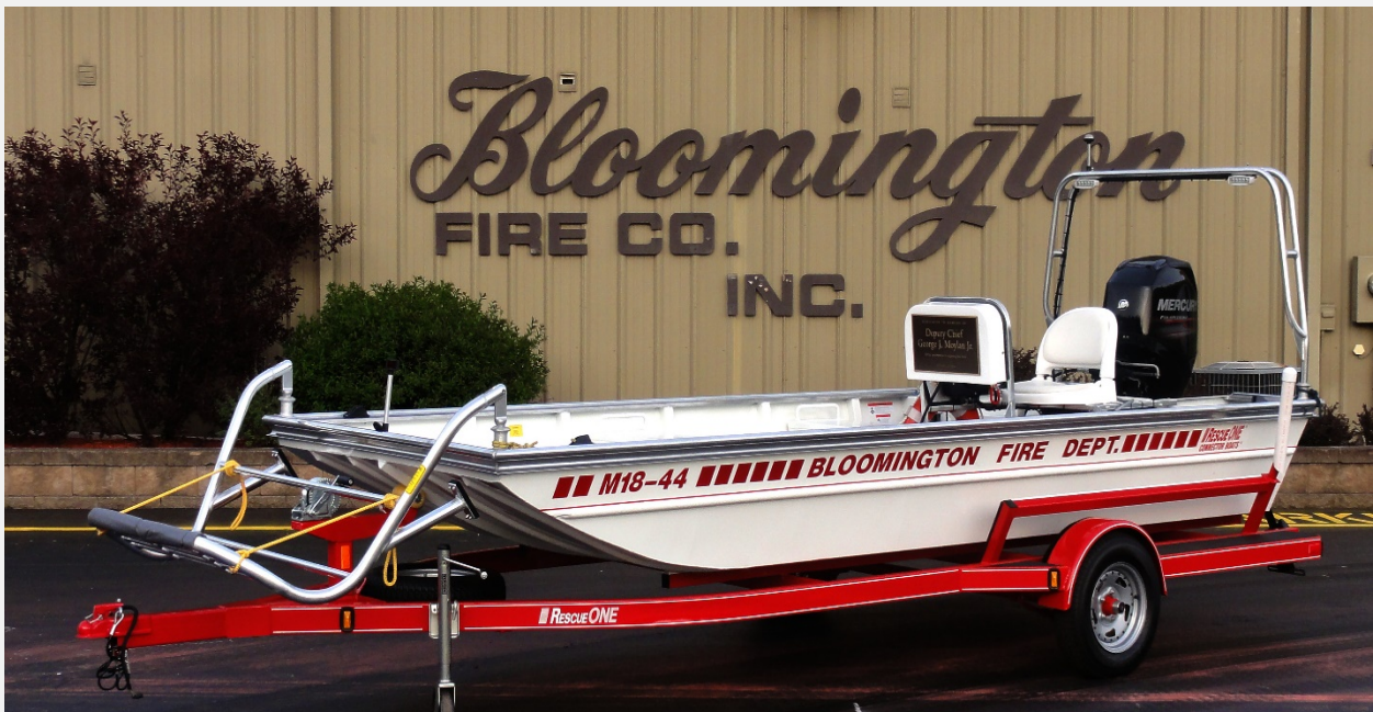
RB-1(M-18-44) - 2014 Rescue One Connector Boat / 40 horse power Mercury Jet Drive Engine with dive platform on front.
