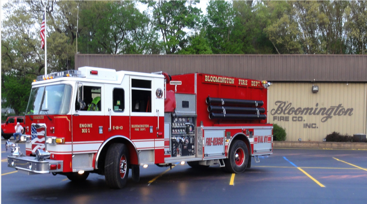
E-18-20 - 2009 Pierce Arrow XT Pumper 6 Passenger Cab, 1500gal/min Waterous pump / 1500gal water tank
