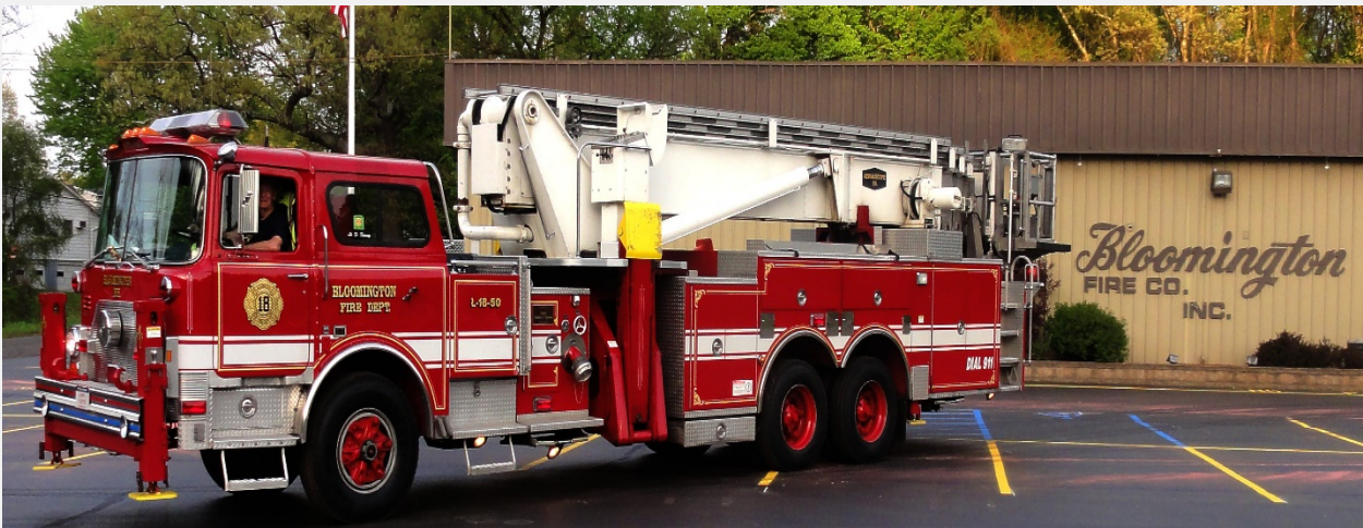
L-1850 – 1996 95' Mack Tower Ladder / 95' aerial scope / 6 passenger cab / refurbished by Pierce in 2002
