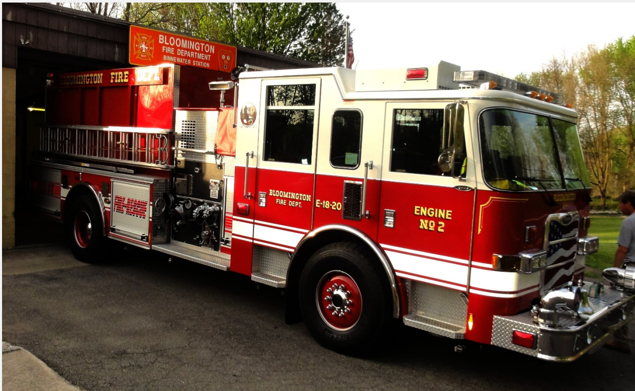
E-18-20 - 2009 Pierce Arrow XT Pumper 6 Passenger Cab, 1500gal/min Waterous pump / 1500gal water tank
