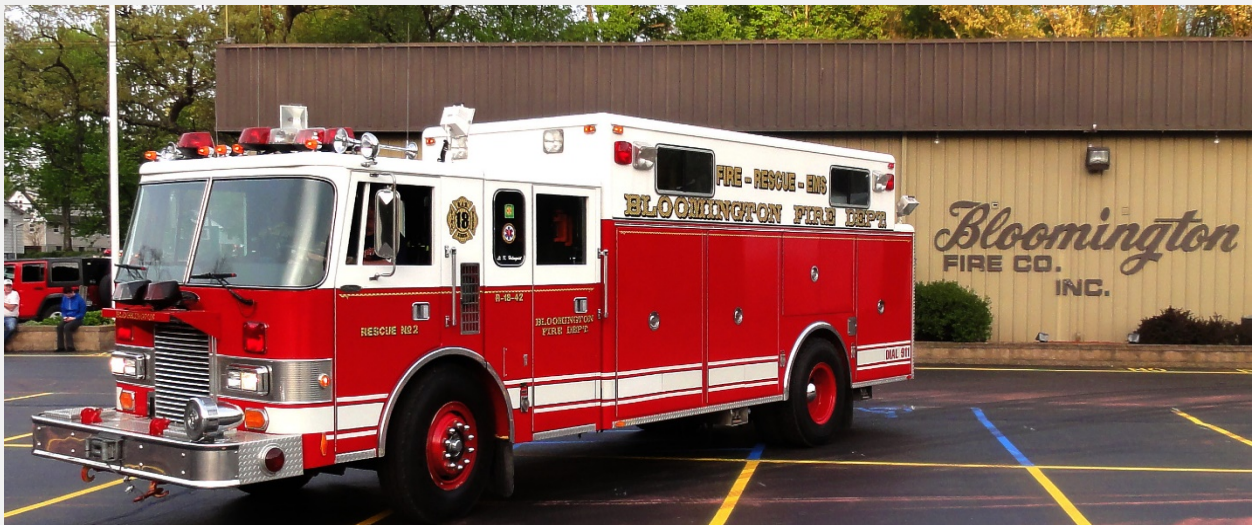
R-18-42 - 1989 Pierce Lance Heavy Rescue/Pumper with Waterous 1000GPM pump.
